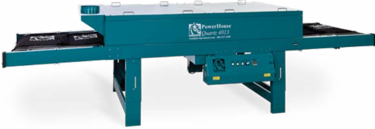
PQ-5217 part 11248 Production: 1,000 + Pieces per Hour Belt Width: 52" (132cm) Dimensions (L x W x H): 204" (518cm) x 60" (158cm) x 32" (81cm) In Feed/Out Feed Dimensions: 60" (132cm) Optional 5' (1.5m) In feed/Out feed Extension Oven Dimensions: 84" (213cm) POWER REQUIREMENTS: Electric: 220-240V, 3-phase, 50-60Hz, 30,600 Watts, 91amps
