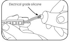
6 CAUTION: Anytime light engine or supply wire is cut and/or wire is exposed, electrical grade silicone must be applied (see list on the next page for recommendations).
