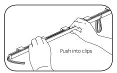
Push each 16 in. (406mm) light engine segment into the clips. Fold loose wires behind light engines.
