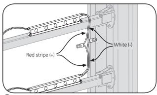
Connect modules using twist-on wire connectors or in-line (IDC) connectors. Join white wires together and red striped wires together.
