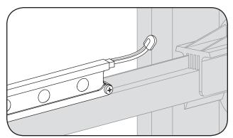
Cap all exposed wires with appropriate end caps or apply electric grade (non-corrosive) silicone for additional weather protection.
