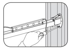
Secure the Mounting Rail to the inside of the box sign using a Tetra® Mounting Rail Bracket or other suitable mounting means. Ensure the #6 (M3) screw does not exceed 3/4 inches (19 mm) in length.
