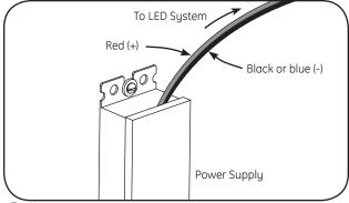
Run a wire from the power supply to inside the sign and connect to the first module on the strip.
