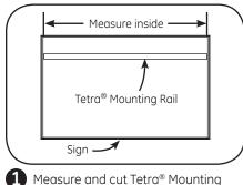
Rail or other suitable mounting means to appropriate length to fit into sign.
