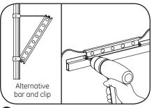
Arrange modules evenly spaced apart. Place the Tetra® modules on the Mounting Rail and secure into lip with a self-tapping #6 (M3) screw or 1/8-inch (3.175 mm) rivet. Or mount using the alternative bar and clip configuration.
