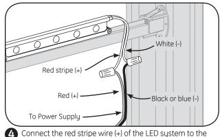
Connect the red stripe wire (+) of the LED system to the red wire (+) of the power supply. Connect the white wire (-) of the LED system to the black or blue wire (-) of the power supply.
