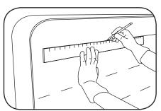
1 Mark row spacing guidelines so that modules are spaced evenly inside and from edges of sign.
