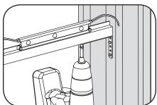
Secure the Mounting Rail to the inside of the box sign using a Tetra<sup>®</sup> Mounting Rail Bracket or other suitable mounting means. Ensure the #6 (M3) screw does not exceed 3/4 inches (19 mm) in length.
