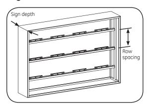
Recommended sign depth is 3-5 in. (76.2 mm-127 mm) for single sided and 6-10 in. (152.4 mm-254 mm) for double sided applications.
