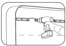
Secure with at least one screw per module with #6 or #8 (M3 or M4) screws or 1/8-inch rivets (3.175 mm), silicone or equivalent.
