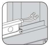
2 Cap all exposed wires with wire nuts or apply electric grade (non-corrosive) silicone for additional weather protection.
