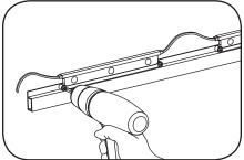
Arrange modules evenly spaced apart. Place the Tetra® modules on the Mounting Rail and secure into lip with a self-tapping #6 (M3) screw or 1/8-inch (3.175 mm) rivet.
