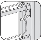
Connect modules using twist-on wire connectors or in-line (IDC) connectors. Join white wires together and red striped wires together.
