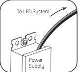
Run a wire from the power supply to connect to the first module on the strip.
