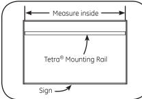
Measure and cut Tetra<sup>®</sup> Mounting Rail or other suitable mounting means to appropriate length to fit into sign.
