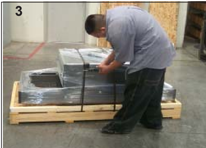
Unband using scissors (Photo 3)., be careful that the band does not spring towards you. Remove the shrink wrap (Photo 4).
