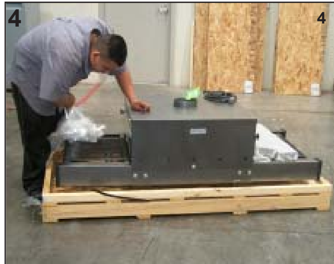
Unband using scissors (Photo 3)., be careful that the band does not spring towards you. Remove the shrink wrap (Photo 4).
