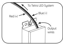
Connect the supply wire that is attached to the Tetra LED System to the red (+) and blue (-) output wires of the power supply as outlined in the "Electrical Connections" section of your LED system's Installation Instructions.
