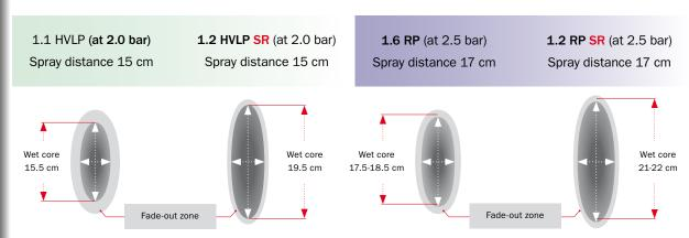
Standard nozzles with wet, compact core. SR nozzles with wide-streched core.
