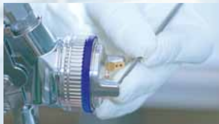
Hand adjustment: Each nozzle set is separately manually "tuned" to optimise the spray fan.
