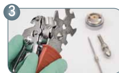
And finally, unscrew fluid tip with the ring spanner integrated in the universal spanner.
