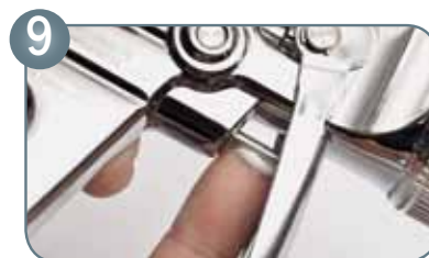
Grease visible part of air piston rod
