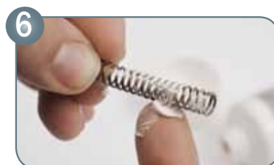
Grease and insert paint needle spring
