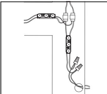
**WARNING:** Connect Red striped wire of LED modules (+) to Red wire of power supply (+). Connect White wire of LED modules (-) to Black wire of power supply (-). Reverse polarity connections may damage LEDs and will void product warranty.
