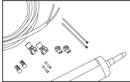
2. **Supplies required:** PLTC cable, wire nuts, IDC connectors or butt splices with appropriate safety agency markings, and cable ties. **Optional:** Screws and silicone.
