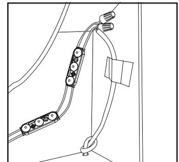
8. **Connect power supply to first module on string:** See power supply install guide for more information regarding power supply installation.
