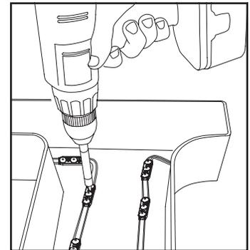
5. **Fasteners:** If desired, modules can be secured with #6 (3.5 mm) pan head sheet metal screws or 3/8 in (3 mm) aluminum rivets. **NOTE: If installing SloanLED Prism Mini, skip to Step 6.**
