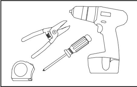
1. **Tools required:** Measuring tape, wire strippers. **Optional:** Drill, screwdriver.
