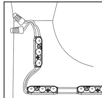
7. **Cap all unused wires:** The strand of modules should not be looped to create a closed circuit.
