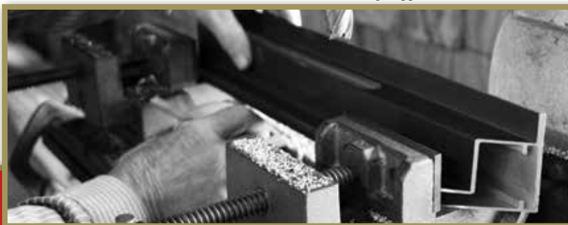
Fabricating Support Arms for Vandal cover
