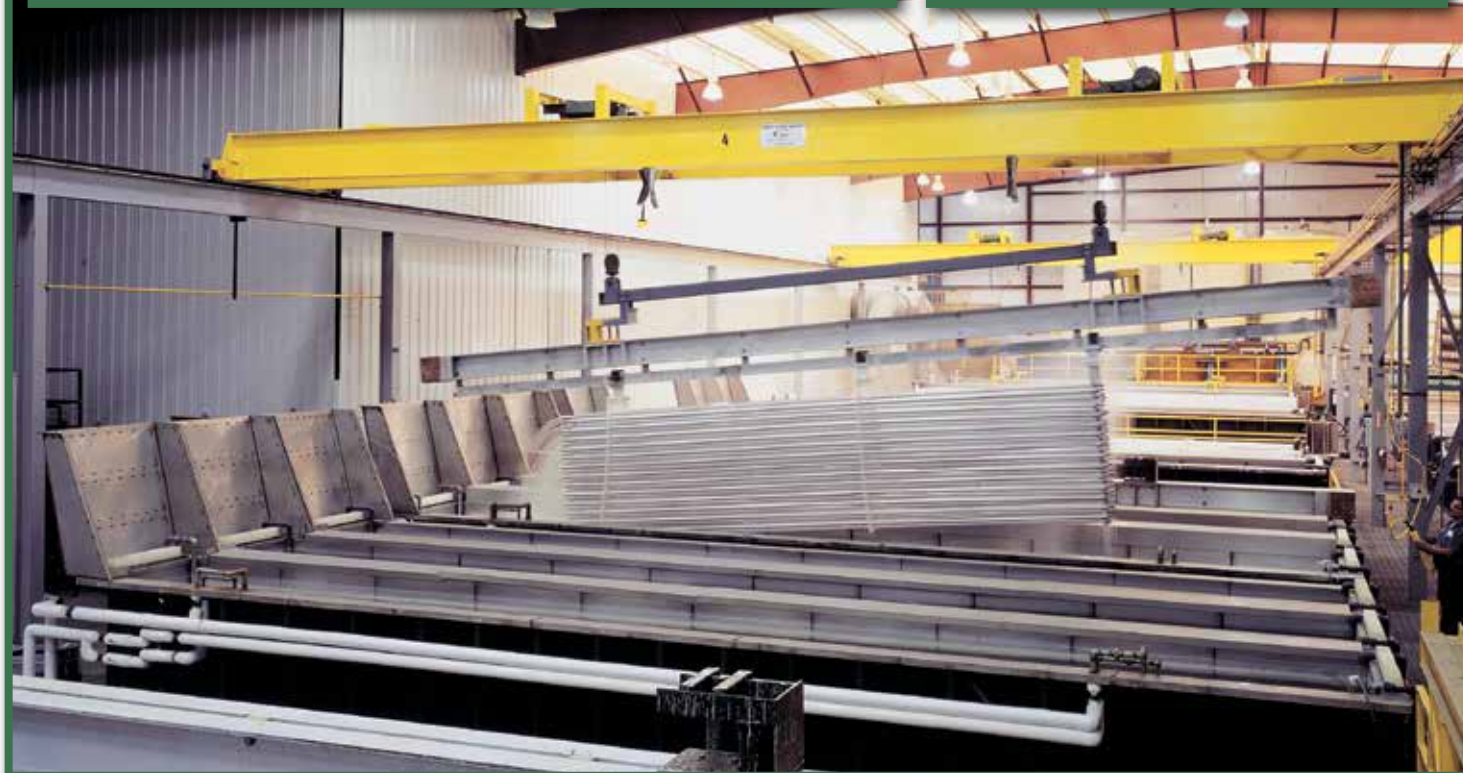
Anodizing bath for full length extrusions
