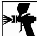
Apply Metallic colors with a spray gun or an aerosol can as needed to obtain opacity. Brush application with metallic colors will not produce the desired appearance.
