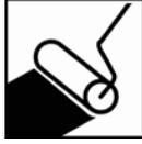
Apply Solid Colors with a small brush or a small foam roller as needed to obtain opacity. Use appropriate solvent resistant brush.
