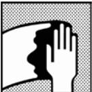
Clean the surface to be sprayed with a 1 to 1 mixture of T-4000 cleaner and Distilled water. Make certain all water spots are removed. Follow this cleaning by wiping with clean and clear water using soft clean cloth or paper towels. Dry the panel completely with the same type of towel. Akzo Nobel Premium Wipes work very well for this cleaning.
