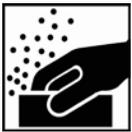
Existing finish should be sanded or scuffed to eliminate surface roughness in the scratch. Avoid sanding to bare metal when possible.
