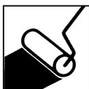
Apply as needed to obtain opacity. Use appropriate solvent resistant roller.
