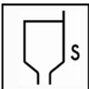
The proper spraying viscosity is achieved by using the recommended mixing ratio. 23–28 sec. ZAHN cup #2 (20–25 sec. DIN cup #4) at 70°F (20°C).
