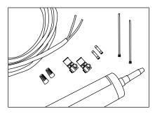
2. Supplies required: Junction box, #8 or #10 pan head screws, UL Listed PLTC cable, electrical wire connectors, ½ in (13 mm) locknuts, silicone
