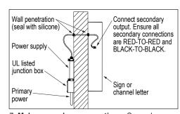
7. Make secondary connections: Secondary class 2 cables do not require conduit per NEC 2008 Articles 725.121 through 725.130. Seal all wall penetrations with silicone to avoid water damage.
