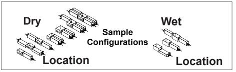
4. Configure Power Supplies: Secure power supplies to junction box using ½ in (13 mm) locknuts. Power supplies may be joined together in a wide array of configurations. For wet locations use a UL Listed for wet locations junction box. For dry locations use any UL Listed junction box.
