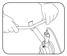
**Part 2:** The workable forming time is about 2–3 minutes. The light guide must remain in the desired position until completely cooled. See the chart above for minimum bend radius guidelines.
