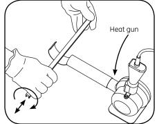
**Part 1:** Move the section back and forth while rotating about the diameter until it is soft and pliable. Gently bend to the desired angle.
