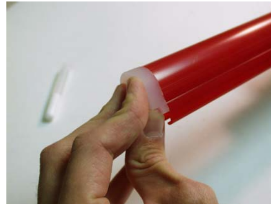
Hold end cap in place with pressure until the glue sets. Approximately 15 seconds. Figure 18
