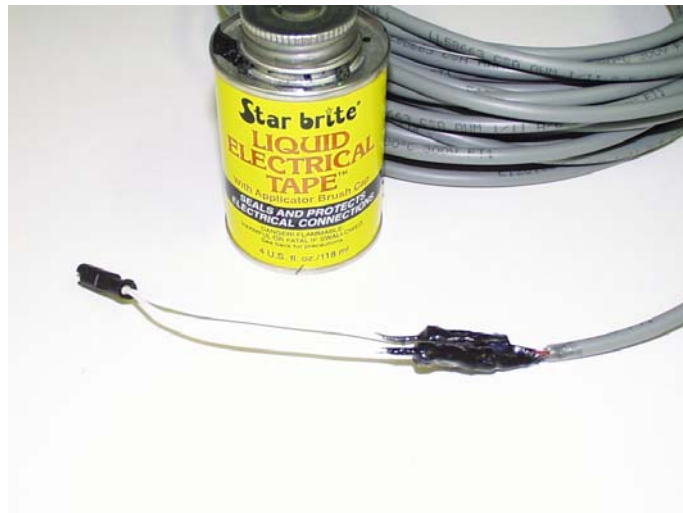
Covering butt splices with liquid electrical tape Figure 27
