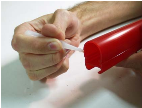
Apply glue around end of cut LEDStripe tube. Figure 17
