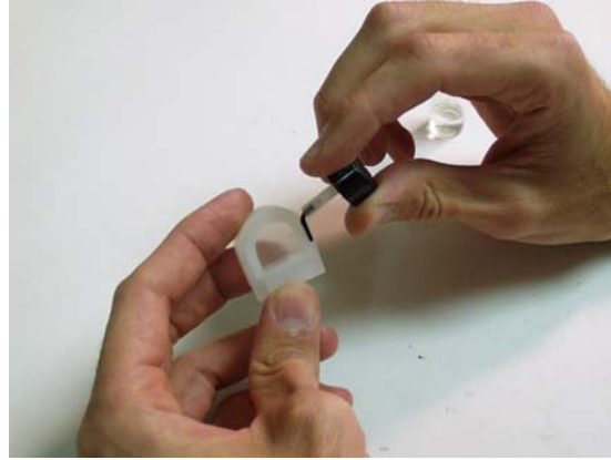
Apply primer all around the edge of the Silicone End Cap. Figure 16
