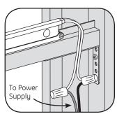
Connect the red stripe wire (+) of the LED system to the red wire (+) of the power supply. Connect the white wire (-) of the LED system to the black or blue wire (-) of the power supply.
