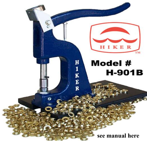
LOAD - Top Die holds grommet firmly.
