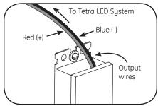
Connect the supply wire that is attached to the Tetra LED System to the red (+) and blue (-) output wires of the power supply as outlined in the "Electrical Connections" section of your LED sustem's Installation Instructions.
